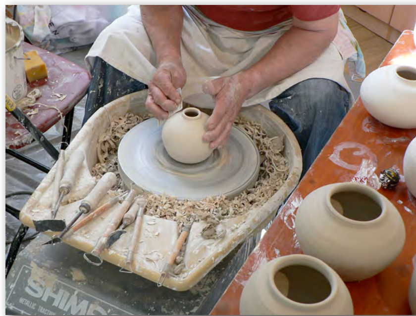
Figure 5.6-18 Pottery is made on a pottery wheel by revolving the clay around a central axis.
